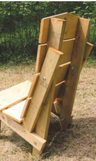
PIC 10. It's not particularly elegant from the back, I admit. I could have softened those 100 x 50mm struts with angled cuts, but this end-grain is the most vulnerable to rot, so I preferred to leave it at a minimum. One step more in decorative detail might be acceptable (like the pointed top plank and the chamfers top and bottom), but detail must be kept in scale and this is, after all, made from sawn tanalised building timber and delights in not being fine cabinetry. (Actually, I don't think I agree with myself. The more I look at this, the more I think four 45° cuts halfway along the top of the struts would improve the back view)
